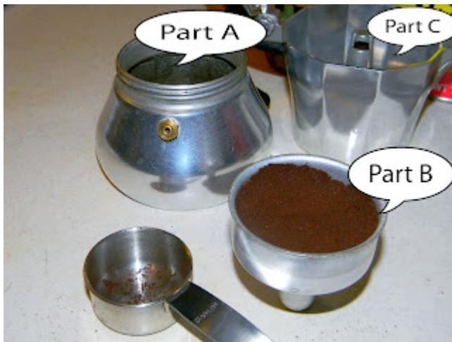
The boiler (marked A) is filled with water almost up to the safety release valve and the funnel shaped metal filter (B) is inserted. Finely-ground coffee is added to the filter.. Then the upper part (C, which has a second metal filter at the bottom) is tightly screwed onto the base.
